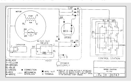
115-1-60 HOISTS WITHOUT CONTACTOR (Orange Control Station)
