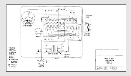
220-3-50 230-3-60 HOISTS WITH CONTACTOR (Black Control Station)
