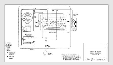
115-1-60 HOISTS WITH CONTACTOR (Black Control Station)
