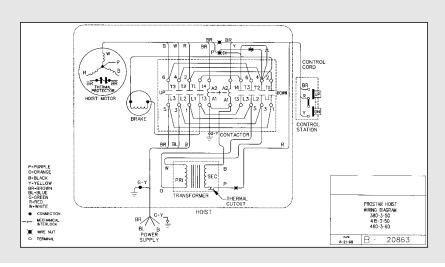
380-3-50 415-3-50 460-3-60 HOISTS WITH CONTACTOR (Black Control Station)
